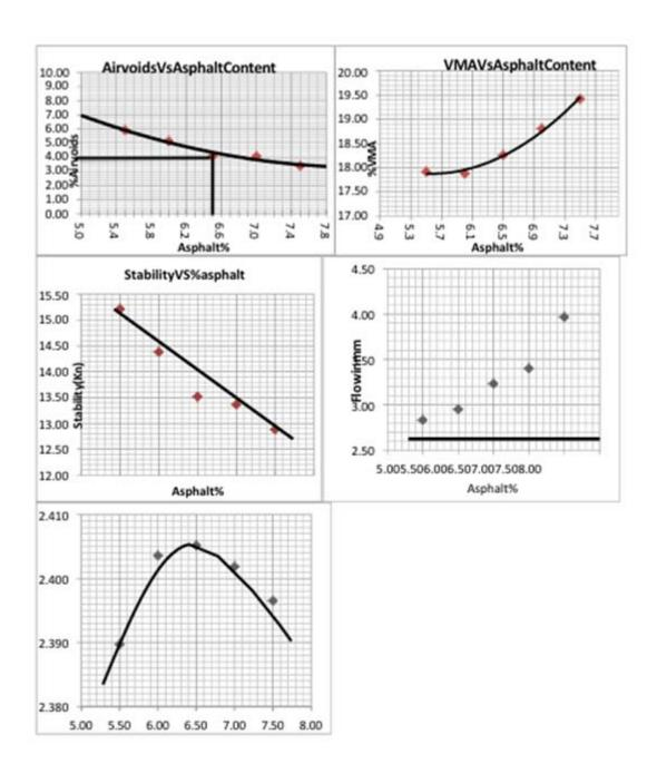
Graphical representation of Marshall Test results with VG40
